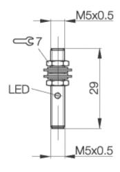
Inductive Sensors BES M05EC-NSC08B-S26G M5x0,5 x 29 normally-open Sn=0,8mm shielded
